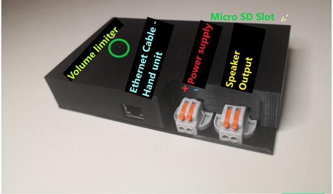
In the top of the Case is an additional hole for limiting the maximum volume(circled green). Default it's all the way up. I do not know why anyone would want to change that, but yeah, I added it nonetheless. If you want to limit it, insert a screwdriver (flat) into the hole and turn it LIGHTLY counterclockwise. Don't rip it off, dumbass.
